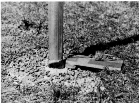
Experimental loading system for using the 40-foot vertical on 75 meters.
