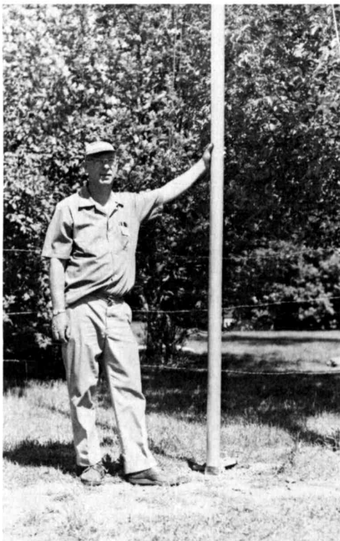
Author W7CSD with his three-band 40-foot irrigation-pipe vertical.
